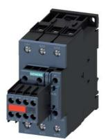
power contactor, AC-3e/AC-3, 80 A, 37 kW / 400 V, 3-pole, 110 V AC, 50 Hz / 120 V, 60 Hz, auxiliary contacts: 2 NO + 2 NC, screw terminal, size: S2, captive auxiliary switch
