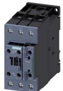
power contactor, AC-3e/AC-3, 80 A, 37 kW / 400 V, 3-pole, 110 V AC, 50 Hz / 120 V, 60 Hz, auxiliary contacts: 1 NO + 1 NC, screw terminal, size: S2  $\,$
