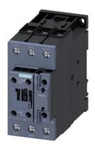
power contactor, AC-3e/AC-3, 80 A, 37 kW / 400 V, 3-pole, 110 V AC, 50 Hz / 120 V, 60 Hz, auxiliary contacts: 1 NO + 1 NC, screw terminal, size: S2, multi-unit packaging, pack = 6 units
