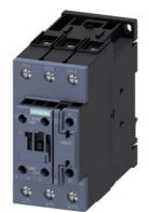
power contactor, AC-3e/AC-3, 80 A, 37 kW / 400 V, 3-pole, 110 V AC, 50 Hz / 120 V, 60 Hz, auxiliary contacts: 1 NO + 1 NC, screw terminal, size: S2, upright mounting position
