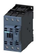
traction contactor, AC-3e/AC-3, 65 A, 30 kW / 400 V, 3-pole, 72 V DC, 0.7-1.25\* Us, electronic drive, with integrated varistor, auxiliary contacts: 1 NO + 1 NC, main circuit: screw terminal, control and auxiliary circuit: spring-loaded terminal, size: S2
