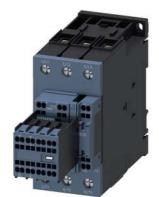
traction contactor, AC-3e/AC-3, 65 A, 30 kW / 400 V, 3-pole, 110 V DC, 0.7-1.25\* Us, electronic drive, with integrated varistor, auxiliary contacts: 2 NO + 2 NC, main circuit: screw terminal, control and auxiliary circuit: spring-loaded terminal, size: S2, removable auxiliary switch
