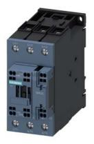
traction contactor, AC-3e/AC-3, 65 A, 30 kW / 400 V, 3-pole, 110 V DC, 0.7-1.25 $^{\star}$  Us, electronic drive, with integrated varistor, auxiliary contacts: 1 NO + 1 NC, main circuit: screw terminal, control and auxiliary circuit: spring-loaded terminal, size: S2
