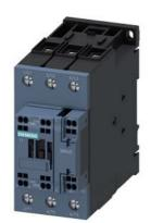
traction contactor, AC-3e/AC-3, 65 A, 30 kW / 400 V, 3-pole, 24 V DC, 0.7-1.25\* Us, electronic drive, with integrated varistor, auxiliary contacts: 1 NO + 1 NC, main circuit: screw terminal, control and auxiliary circuit: spring-loaded terminal, size: S2
