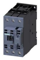
power contactor, AC-3e/AC-3, 65 A, 30 kW / 400 V, 3-pole, 400 V AC, 50 Hz, auxiliary contacts: 1 NO + 1 NC, main circuit: screw terminal, control and auxiliary circuit: spring-loaded terminal, size: S2
