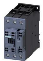
power contactor, AC-3e/AC-3, 65 A, 30 kW / 400 V, 3-pole, 220 V AC, 50/60 Hz, auxiliary contacts: 1 NO + 1 NC, main circuit: screw terminal, control and auxiliary circuit: spring-loaded terminal, size: S2
