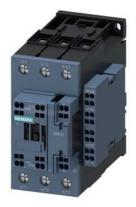
power contactor, AC-3e/AC-3, 65 A, 30 kW / 400 V, 3-pole, 110 V AC, 50 Hz, auxiliary contacts: 2 NO + 2 NC, main circuit: screw terminal, control and auxiliary circuit: spring-loaded terminal, size: S2, lateral auxiliary switch
