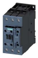
traction contactor, AC-3e/AC-3, 65 A, 30 kW / 400 V, 3-pole, 110 V DC, 0.7-1.25  $^{\star}$  Us, electronic drive, with integrated varistor, auxiliary contacts: 1 NO + 1 NC, screw terminal, size: S2
