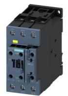
power contactor, AC-3e/AC-3, 65 A, 30 kW / 400 V, 3-pole, 175-280 V AC/DC, 50/60 Hz, with integrated varistor, auxiliary contacts: 1 NC, screw terminal, size: S2, F-PLC-IN
