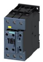
power contactor, AC-3e/AC-3, 65 A, 30 kW / 400 V, 3-pole, 21-33 V AC/DC, 50/60 Hz, with integrated varistor, auxiliary contacts: 1 NC, screw terminal, size: S2, F-PLC-IN
