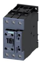
power contactor, AC-3e/AC-3, 65 A, 30 kW / 400 V, 3-pole, 175-280 V AC/DC, 50/60 Hz, with integrated varistor, auxiliary contacts: 1 NO + 1 NC, screw terminal, size: S2
