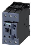
power contactor, AC-3e/AC-3, 65 A, 30 kW / 400 V, 3-pole, 48-80 V AC/DC, 50/60 Hz, with integrated varistor, auxiliary contacts: 1 NO + 1 NC, screw terminal, size: S2
