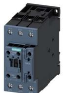
power contactor, AC-3e/AC-3, 65 A, 30 kW / 400 V, 3-pole, 20-33 V AC/DC, 50/60 Hz, with integrated varistor, auxiliary contacts: 1 NO + 1 NC, screw terminal, size: S2, communication-capable
