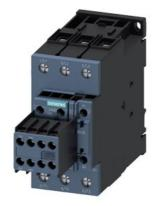
power contactor, AC-3e/AC-3, 65 A, 30 kW / 400 V, 3-pole, 24 V DC, 0.8-1.2\* Us, with integrated varistor, auxiliary contacts: 2 NO + 2 NC, screw terminal, size: S2, suitable for PLC outputs
