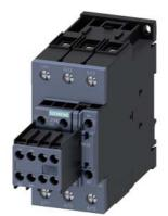
power contactor, AC-3e/AC-3, 65 A, 30 kW / 400 V, 3-pole, 220 V AC, 50 Hz / 240 V, 60 Hz, auxiliary contacts: 2 NO + 2 NC, screw terminal, size: S2, removable auxiliary switch
