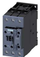
power contactor, AC-3e/AC-3, 65 A, 30 kW / 400 V, 3-pole, 220 V AC, 50 Hz / 240 V, 60 Hz, auxiliary contacts: 1 NO + 1 NC, screw terminal, size: S2  $\,$
