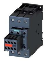
power contactor, AC-3e/AC-3, 65 A, 30 kW / 400 V, 3-pole, 230 V AC, 50 Hz, auxiliary contacts: 2 NO + 2 NC, screw terminal, size: S2, captive auxiliary switch
