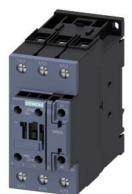
power contactor, AC-3e/AC-3, 65 A, 30 kW / 400 V, 3-pole, 230 V AC, 50 Hz, auxiliary contacts: 1 NO + 1 NC, screw terminal, size: S2, upright mounting position
