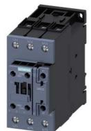
power contactor, AC-3e/AC-3, 65 A, 30 kW / 400 V, 3-pole, 200 V AC, 50 Hz / 200-220 V, 60 Hz, auxiliary contacts: 1 NO + 1 NC, screw terminal, size: S2  $\,$
