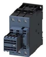
traction contactor, AC-3e/AC-3, 51 A, 22 kW / 400 V, 3-pole, 110 V DC, 0.7-1.25\* Us, electronic drive, with integrated varistor, auxiliary contacts: 2 NO + 2 NC, main circuit: screw terminal, control and auxiliary circuit: spring-loaded terminal, size: S2, removable auxiliary switch
