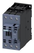
power contactor, AC-3e/AC-3, 51 A, 22 kW / 400 V, 3-pole, 175-280 V AC/DC, 50/60 Hz, with integrated varistor, auxiliary contacts: 1 NO + 1 NC, main circuit: screw terminal, control and auxiliary circuit: spring-loaded terminal, size: S2,
