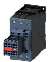
power contactor, AC-3e/AC-3, 51 A, 22 kW / 400 V, 3-pole, 24 V DC, 0.8-1.2\* Us, with integrated varistor, auxiliary contacts: 2 NO + 2 NC, main circuit: screw terminal, control and auxiliary circuit: spring-loaded terminal, size: S2, suitable for PLC outputs, captive auxiliary switch
