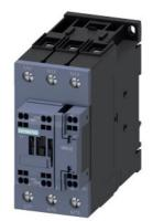
power contactor, AC-3e/AC-3, 51 A, 22 kW / 400 V, 3-pole, 24 V DC, 0.8-1.2\* Us, with integrated varistor, auxiliary contacts: 1 NO + 1 NC, main circuit: screw terminal, control and auxiliary circuit: spring-loaded terminal, size: S2, suitable for PLC outputs
