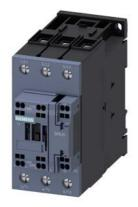
power contactor, AC-3e/AC-3, 51 A, 22 kW / 400 V, 3-pole, 220 V AC, 50/60 Hz, auxiliary contacts: 1 NO + 1 NC, main circuit: screw terminal, control and auxiliary circuit: spring-loaded terminal, size: S2
