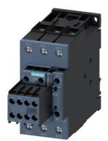
power contactor, AC-3e/AC-3, 51 A, 22 kW / 400 V, 3-pole, 175-280 V AC/DC, 50/60 Hz, with integrated varistor, auxiliary contacts: 2 NO + 2 NC, screw terminal, size: S2, removable auxiliary switch
