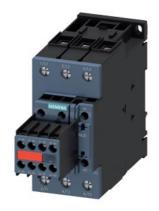
power contactor, AC-3e/AC-3, 51 A, 22 kW / 400 V, 3-pole, 20-33 V AC/DC, 50/60 Hz, with integrated varistor, auxiliary contacts: 2 NO + 2 NC, screw terminal, size: S2, captive auxiliary switch
