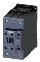
power contactor, AC-3e/AC-3, 51 A, 22 kW / 400 V, 3-pole, 20-33 V AC/DC, 50/60 Hz, with integrated varistor, auxiliary contacts: 1 NO + 1 NC, screw terminal, size: \$52
