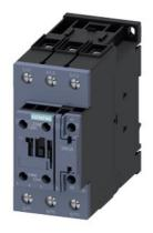
power contactor, AC-3e/AC-3, 51 A, 22 kW / 400 V, 3-pole, 20-33 V AC/DC, 50/60 Hz, with integrated varistor, auxiliary contacts: 1 NO + 1 NC, screw terminal, size: S2, upright mounting position
