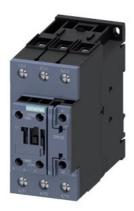
contactor, NEMA version, 25 HP, 460 / 575 V, 3-pole, 20-33 V AC/DC, 50/60 Hz, with integrated varistor, auxiliary contacts: 1 NO + 1 NC, screw terminal, size: S2  $\,$
