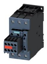
power contactor, AC-3e/AC-3, 51 A, 22 kW / 400 V, 3-pole, 24 V DC, 0.8-1.2\* Us, with integrated varistor, auxiliary contacts: 2 NO + 2 NC, screw terminal, size: S2, suitable for PLC outputs, captive auxiliary switch
