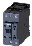
power contactor, AC-3e/AC-3, 51 A, 22 kW / 400 V, 3-pole, 480 V AC, 60 Hz, auxiliary contacts: 1 NO + 1 NC, screw terminal, size: S2
