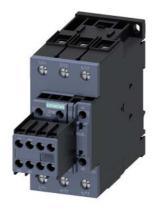
power contactor, AC-3e/AC-3, 51 A, 22 kW / 400 V, 3-pole, 400 V AC, 50 Hz / 400-440 V, 60 Hz, auxiliary contacts: 2 NO + 2 NC, screw terminal, size: S2, removable auxiliary switch
