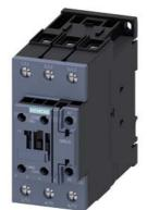
power contactor, AC-3e/AC-3, 51 A, 22 kW / 400 V, 3-pole, 400 V AC, 50 Hz / 400-440 V, 60 Hz, auxiliary contacts: 1 NO + 1 NC, screw terminal, size: S2  $\,$
