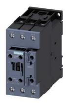
power contactor, AC-3e/AC-3, 51 A, 22 kW / 400 V, 3-pole, 230 V AC, 50 Hz, auxiliary contacts: 1 NO + 1 NC, screw terminal, size: S2, upright mounting position
