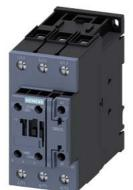
contactor, NEMA version, 25 HP, 460 / 575 V, 3-pole, 110 V AC, 50 Hz / 120 V, 60 Hz, auxiliary contacts: 1 NO + 1 NC, screw terminal, size: S2  $\,$
