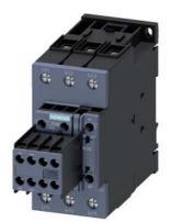
power contactor, AC-3e/AC-3, 51 A, 22 kW / 400 V, 3-pole, 110 V AC, 50/60 Hz, auxiliary contacts: 2 NO + 2 NC, screw terminal, size: S2, removable auxiliary switch
