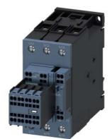
traction contactor, AC-3e/AC-3, 41 A, 18.5 kW / 400 V, 3-pole, 110 V DC, 0.7-1.25\* Us, electronic drive, with integrated varistor, auxiliary contacts: 2 NO + 2 NC, main circuit: screw terminal, control and auxiliary circuit: spring-loaded terminal, size: S2, removable auxiliary switch
