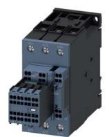
traction contactor, AC-3e/AC-3, 41 A, 18.5 kW / 400 V, 3-pole, 24 V DC, 0.7-1.25\* Us, electronic drive, with integrated varistor, auxiliary contacts: 2 NO + 2 NC, main circuit: screw terminal, control and auxiliary circuit: spring-loaded terminal, size: S2, removable auxiliary switch
