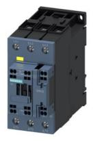
power contactor, AC-3e/AC-3, 41 A, 18.5 kW / 400 V, 3-pole, 175-280 V AC/DC, 50/60 Hz, with integrated varistor, auxiliary contacts: 1 NC, main circuit: screw terminal, control and auxiliary circuit: spring-loaded terminal, size: S2, F-PLC-IN
