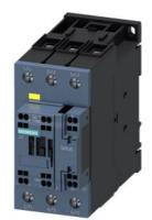
power contactor, AC-3e/AC-3, 41 A, 18.5 kW / 400 V, 3-pole, 83-150 V AC/DC, 50/60 Hz, with integrated varistor, auxiliary contacts: 1 NC, main circuit: screw terminal, control and auxiliary circuit: spring-loaded terminal, size: S2, F-PLC-IN
