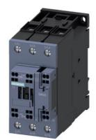
power contactor, AC-3e/AC-3, 41 A, 18.5 kW / 400 V, 3-pole, 175-280 V AC/DC, 50/60 Hz, with integrated varistor, auxiliary contacts: 1 NO + 1 NC, main circuit: screw terminal, control and auxiliary circuit: spring-loaded terminal, size: S2,
