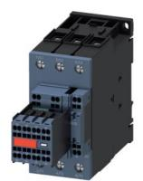
power contactor, AC-3e/AC-3, 41 A, 18.5 kW / 400 V, 3-pole, 20-33 V AC/DC, 50/60 Hz, with integrated varistor, auxiliary contacts: 2 NO + 2 NC, main circuit: screw terminal, control and auxiliary circuit: spring-loaded terminal, size: S2, captive auxiliary switch
