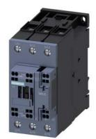
power contactor, AC-3e/AC-3, 41 A, 18.5 kW / 400 V, 3-pole, 220 V AC, 50 Hz / 240 V, 60 Hz, auxiliary contacts: 1 NO + 1 NC, main circuit: screw terminal, control and auxiliary circuit: spring-loaded terminal, size: S2
