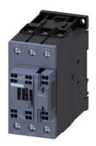
power contactor, AC-3e/AC-3, 41 A, 18.5 kW / 400 V, 3-pole, 230 V AC, 50/60 Hz, auxiliary contacts: 1 NO + 1 NC, main circuit: screw terminal, control and auxiliary circuit: spring-loaded terminal, size: S2, upright mounting position
