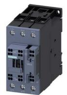
power contactor, AC-3e/AC-3, 41 A, 18.5 kW / 400 V, 3-pole, 110 V AC, 50/60 Hz, auxiliary contacts: 1 NO + 1 NC, main circuit: screw terminal, control and auxiliary circuit: spring-loaded terminal, size: S2
