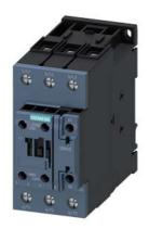
traction contactor, AC-3e/AC-3, 41 A, 18.5 kW / 400 V, 3-pole, 24 V DC, 0.7-1.25  $^{\ast}$  Us, electronic drive, with integrated varistor, auxiliary contacts: 1 NO + 1 NC, screw terminal, size: S2
